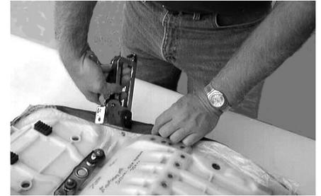
Continue working your way around the seat by applying even pressure and installing staples one to two inches apart. Periodically turn the seat cover over and check for straightness until entire seat cover is securely installed.
